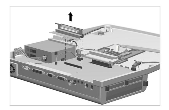
Figure 7-14. Removing the MPEG Connector
